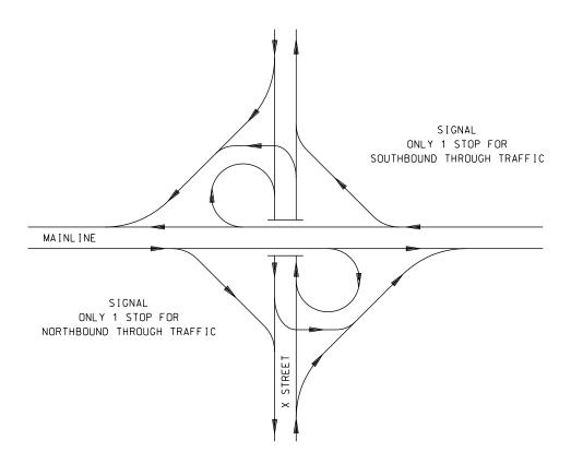
PARCLO B – 4 QUAD. (ONE EXIT LOOP, ONE EXIT RAMP, ENTRANCE RAMPS) Figure 6-1.03I
