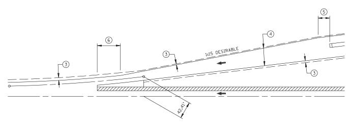
METERED RAMP AND H.O.V. BYPASS MERGE AREA DESIGN
