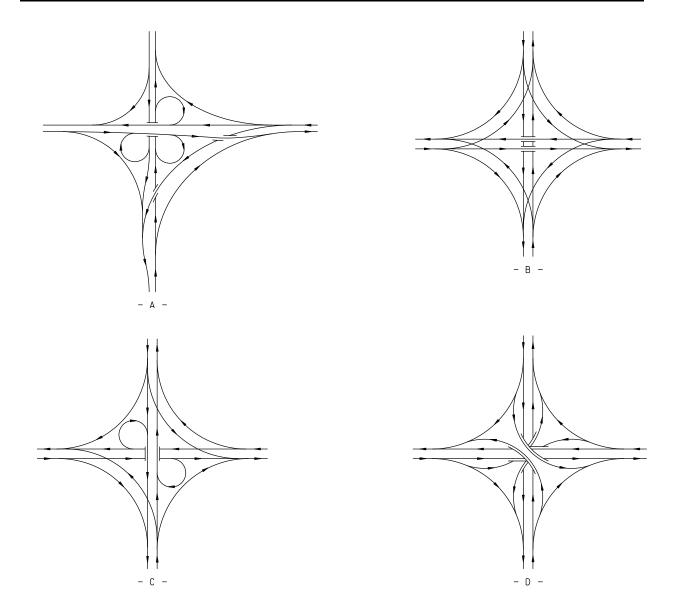
DIRECTIONAL AND FULLY-DIRECTIONAL INTERCHANGES Figure 6-1.03L
