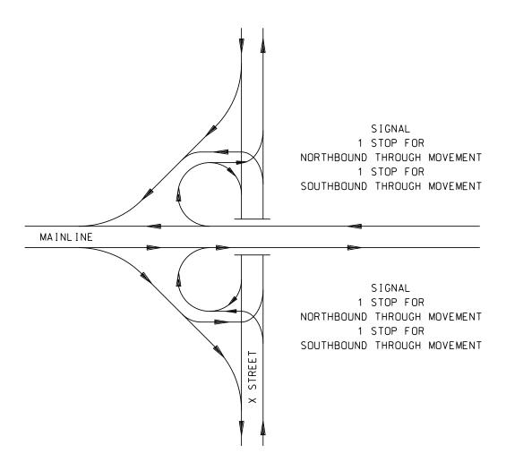
PARCLO AB/FOLDED DIAMOND (ONE EXIT LOOP, ONE EXIT RAMP, ONE ENTRANCE LOOP, ONE ENTRANCE RAMP) Figure 6-1.03J
