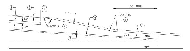
SYSTEM TO SYSTEM RAMP H.O.V. BYPASS DESIGN
