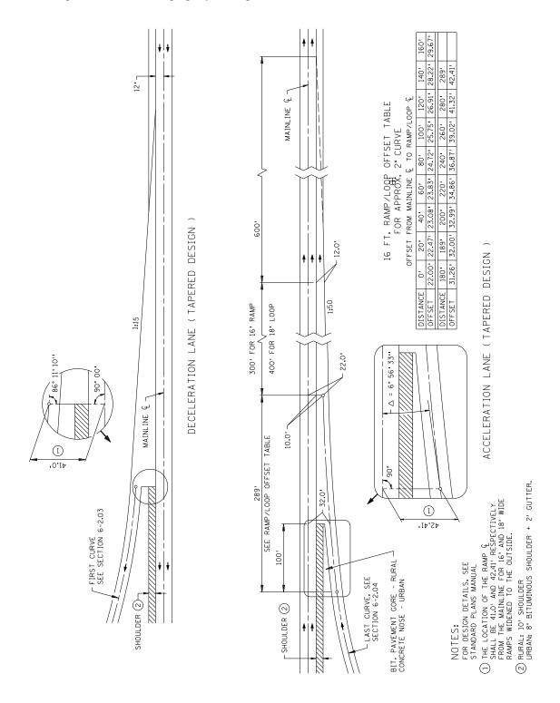
ACCELERATION AND DECELERATION LANES, MAINLINE TANGENT SECTION TAPERED DESIGN
