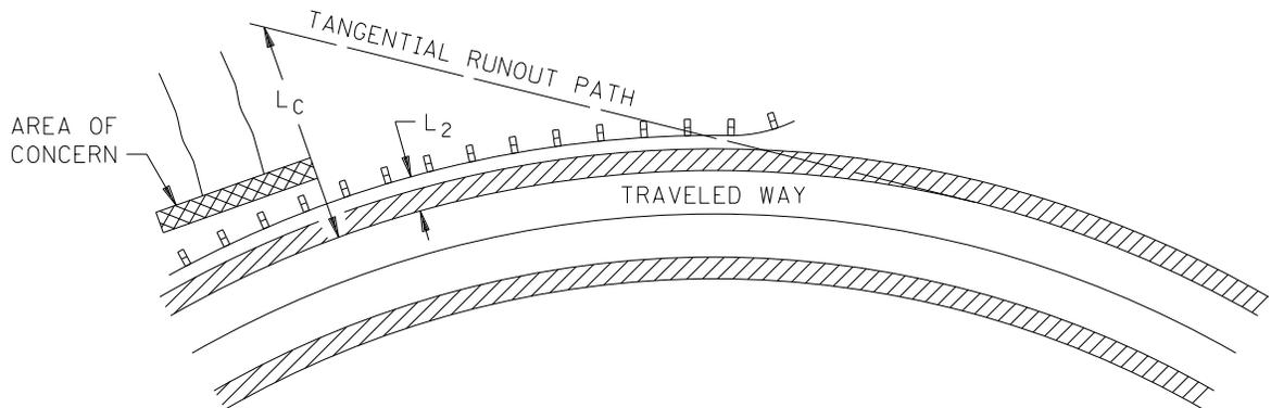
**EXAMPLE OF BARRIER DESIGN FOR FIXED OBJECT ON HORIZONTAL CURVE**
