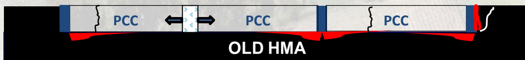
Figure 1. Water in joints can lead to reduced layer bonding, erosion, cracking, and panel shifting (ice expansion)
